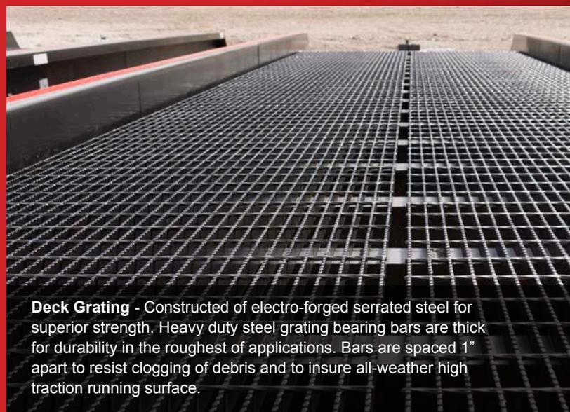
**Deck Grating** - Constructed of electro-forged serrated steel for superior strength. Heavy duty steel grating bearing bars are thick for durability in the roughest of applications. Bars are spaced 1" apart to resist clogging of debris and to insure all-weather high traction running surface.
