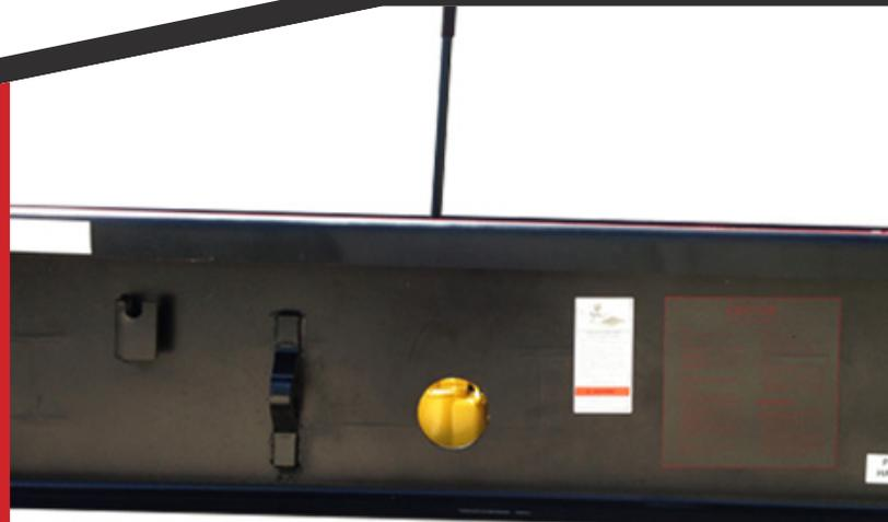
**Pump** - Hydraulic hand pump quickly adjusts top end of ramp with the bed of the vehicle or loading dock. The handle is stored out of the way when not in use.
