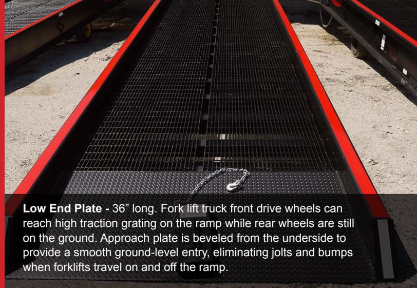
**Low End Plate** - 36" long. Fork lift truck front drive wheels can reach high traction grating on the ramp while rear wheels are still on the ground. Approach plate is beveled from the underside to provide a smooth ground-level entry, eliminating jolts and bumps when forklifts travel on and off the ramp.
